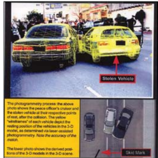
An example of laser-assisted photogrammetry.
